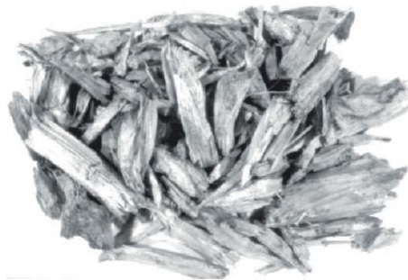
b) Hog fuel (crushed with blunt tools)
