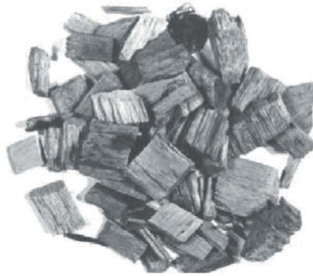
a) Wood chips (cut with sharp tools)
